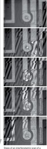
Steps of an interferometric scan of a wafer surface
