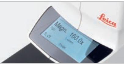
The digital display of the Leica M205 A shows all essential settings at a glance
