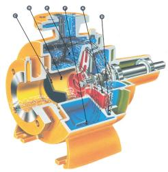
If for some reason, air penetrates into the suction pipe and the pump stops pumping, the priming process starts again as described above, and continues until normal pumping has been resumed
