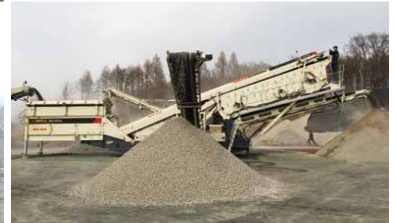
NFS350's application of the screening of finished hard rock and aggregate
