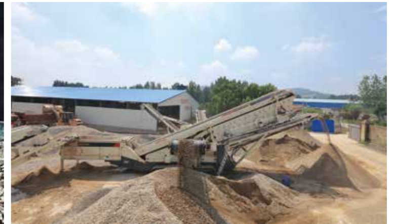
NFS350's application of the screening of the gravel and aggregate from the road and bridge construction in Shandong Province
