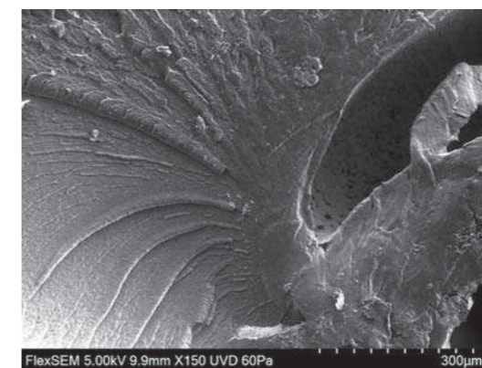
FlexSEM 5.00kV 9.9mm X150 UVD 60Pa Accelerating voltage: 5.0 kV, Magnification: 150x Signal: UVD-II Specimen: resin fracture
