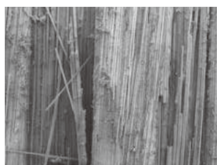
Low accelerating voltage SE image Sample: CFRP
