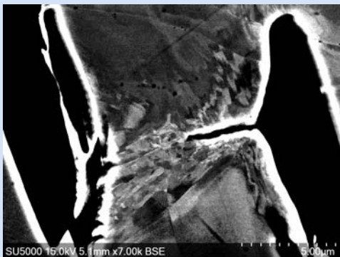
Sample: Heat resistant steel Vacc: 15 kV New 5-segment PD-BSE demonstrating high orientation contrast image at low take-off angle (left). The correlative grain misorientation map acquired through EBSD (right), showing contrast precision corresponding to 0.5 degree misorientation.
