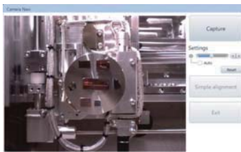
Left: Picture of the specimen captured by the camera equipped inside the chamber. Right: Camera image transferred to the SEM MAP screen for navigation.
