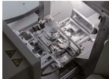
Right: external view of the stage. XY movable range: 135 x 100 mm
