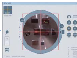
Left: Picture of the specimen captured by the camera equipped inside the chamber. Right: Camera image transferred to the SEM MAP screen for navigation.
