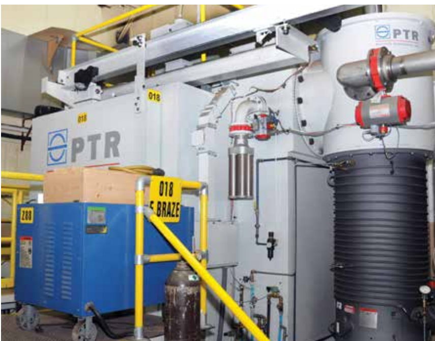
Large EBrace welding machine located at the Dresser-Rand facility in Olean, NY.
