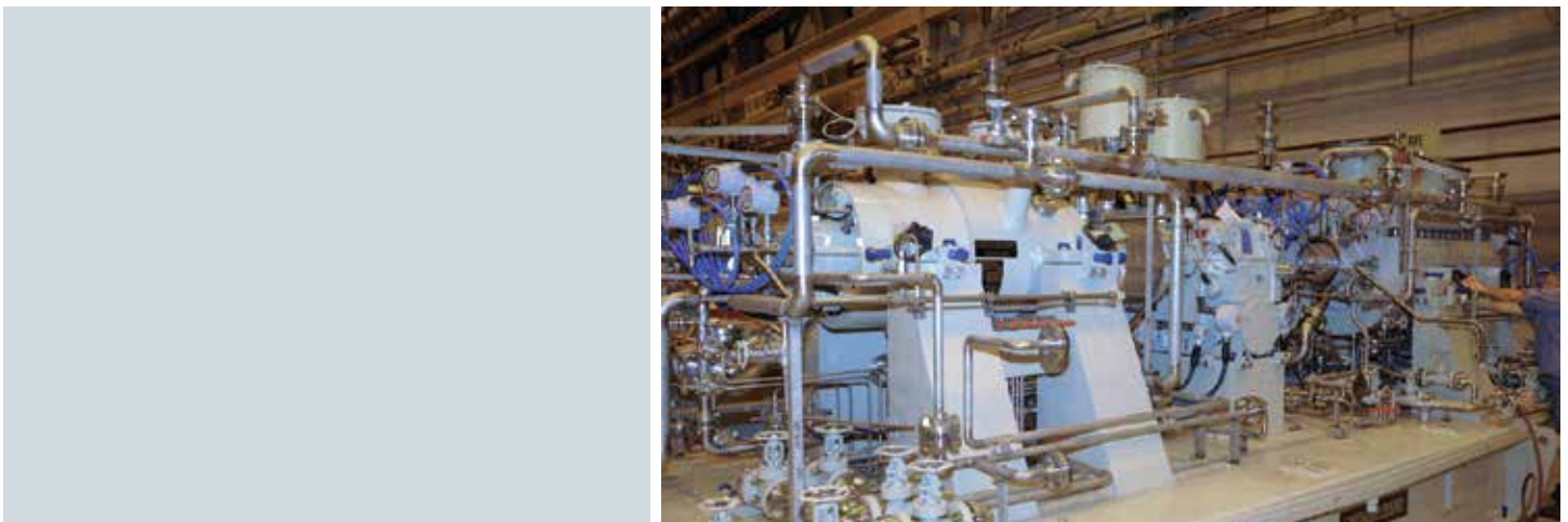
A D4 DATUM® compressor being assembled at the D-R facility in Olean, NY.
