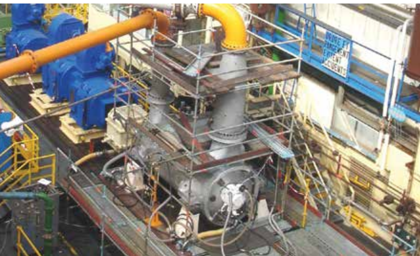
DATUM model D18R9S (destined for hydrogen service in a Spanish refinery) on test stand in Le Havre, France. The Le Havre test facility allows for full load testing of compressor trains, together with their gas turbine or electric motor drivers.
