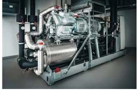
Heat pumps are designed to produce hot water at a specified temperature. Heat is extracted from a low-temperature source such as air, ground water, or waste process heat, and its temperature is raised to a higher level by means of a refrigeration cycle, where it can be used for a heating applications.
