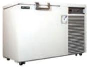
The CRYO freezer -150°C is perfect for long term preservation of for example cells and tissues. The CRYO freezer features a dual cooling system, which consists of two independent systems, offering you the best security for your samples. If one of the refrigeration systems should fail, the other refrigeration system will keep the temperature at -130°C until service is provided.
