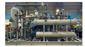
Refrigerant Gas Compressor, Screw type API 619, building more than 3000 screw block per year, Halocarbons, Hydrocarbons, NH3 and C02, 600 psig DWP, slide valve capacity control, variable volume ratio (Vi), Differential pressure lube system, Anti-friction bearings, Micro-panel / PLC control, 676 to 6500 cfm.
